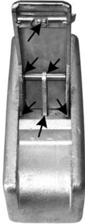
FIGURE 6: COUPLER LUBRICATION POINTS
